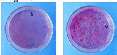
Figure 1. Bacterial (*E. coli*) sensitivity against ZnOa-set (left) and ZnO4-set (right) tetrapods (20 mg/ml) with 100% and 27% reduction of the bacteria viability correspondently.
