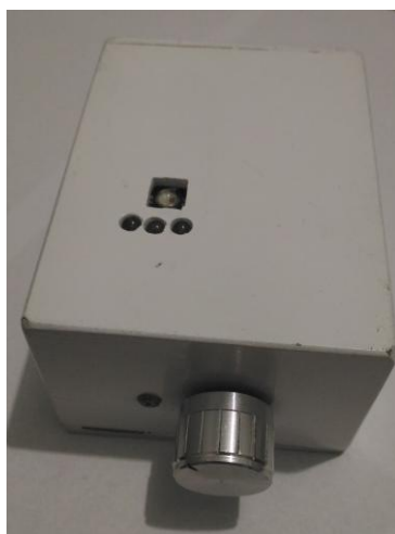
Figure 2. Device for studying skin reaction to light
